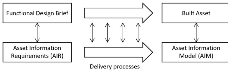
**Figure 2.1: Parallel delivery of built asset and asset data**
